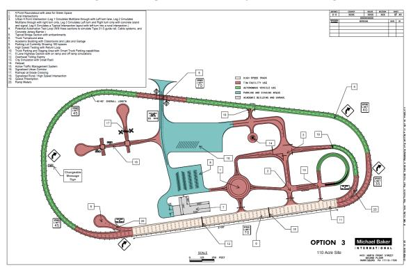
Figure 3: Site Plan for PennSTART training facility at State College, PA. (Courtesy of the Pennsylvania Turnpike Commission.)
